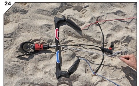
24 Pull line #5 and the Flag Out Line back through the chickenloop and bar.
