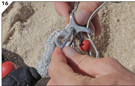
16 Wind the screw back in, ensuring the screw goes through the loop.
